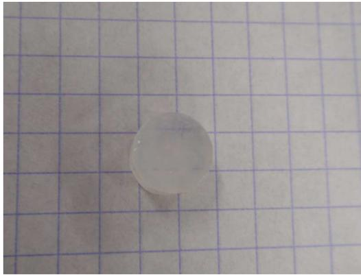
Fig. 1. A photograph of the grown CsI:Na,  $^{133}\text{Ba}$  crystal.
