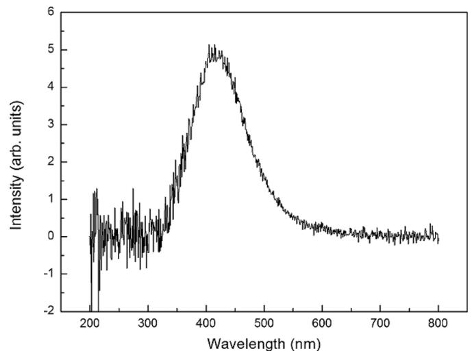
Fig. 2. X-ray induced emission spectrum of the CsI:Na,  $^{133}\text{Ba}$  crystal. The peak wavelength of CsI:Na,  $^{133}\text{Ba}$  crystal was approximately 420 nm.
