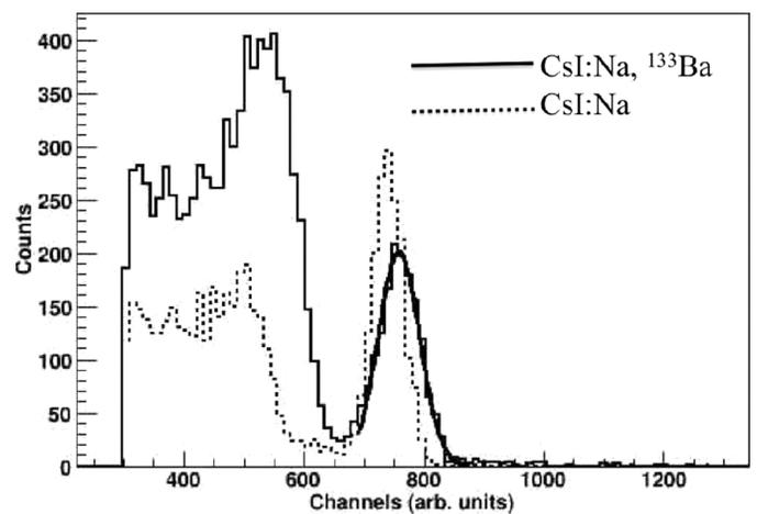
Fig. 3. It shows the energy resolution and relative light yield of the CsI:Na,  $^{133}\text{Ba}$  crystal (solid line) for 662 keV from  $^{137}\text{Cs}$  radioactive source. Dotted line shows pulse height spectrum of the CsI:Na crystal for 662 keV from  $^{137}\text{Cs}$  radioactive source. The energy resolution of CsI:Na,  $^{133}\text{Ba}$  crystal was 10% (FWHM).
