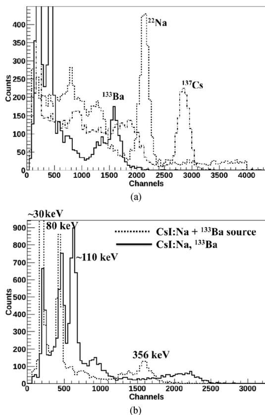
Fig. 6. (a) Pulse height spectrum of the CsI:Na crystal for various  $\gamma$ -ray source such as 356 keV from  $^{133}\text{Ba}$  (solid line), 511 keV from  $^{22}\text{Na}$  (dotted line) and 662 keV from  $^{137}\text{Cs}$  (dash-dotted line). (b) Comparison of the internal radioactivity decay spectrum of CsI:Na,  $^{133}\text{Ba}$  crystal with an energy spectrum of CsI:Na crystal irradiated with  $^{133}\text{Ba}$  radioactive source.
